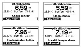
Problems which arise during calibration can have different sources: the sensor, measuring temperature, buffer solutions etc. Special note should be taken of the symptoms of the problem as these are useful for locating the source of the problem.
