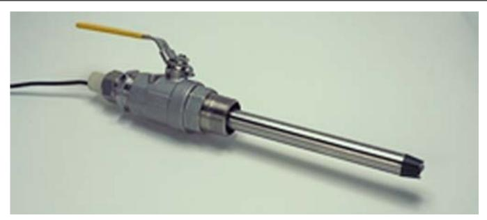
The LiveTap™ Insertion Assembly is ideal for use in areas where down time is critical by allowing removal of the electrode from a live line or tank without process interuption. Fitted with a 1.5" ball valve, the pH or ORP electrode can be removed for maintenance by sliding the 316L Stainless Steel sheath through the valve and closing it off. Your unit is now safe to remove.
