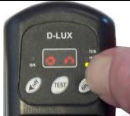
When the unit is installed correctly and operational, you can change the pre-set values to anything ranging from 0.1 sec to 99 hrs.
