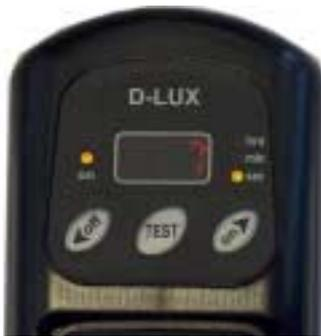
The D-Lux will start with its pre-set time setting of 10 sec ON and 30 sec OFF.
