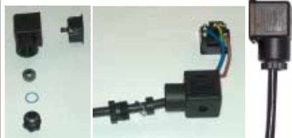
Remove the protection cap from the connector and connect your power cable as shown
