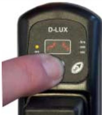
You can press the TEST button anytime to check the valve operation or to manually activate the valve to discharge any condensate. When the test (middle) button is pressed a flowing pattern is displayed indicating the test function is in process.
