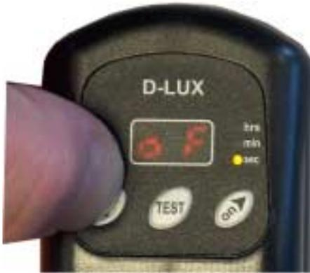
To change the OFF time simply press the left 'off/arrow down' button and 'of' will appear briefly on the display.
