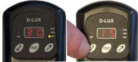
The previously set OFF time will appear on the display (30) and the sec led will be on. You can now press the left 'off/arrow down' button for decreasing the time or the right 'on/arrow up' button to increase the time. The sec, min or hrs led will highlight the time bracket (i.e 1-99 sec or 1-99 min or 1-99 hrs)
